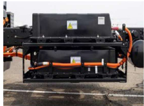
The battery, of the highest water tightness grade of IP68, is positioned 240 mm above the ground surface to prevent water contact and any associated failures.
