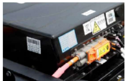
Watertightness Grade IP68, advanced watertightness that prevents any entry of dust and moisture, of a level that keeps the battery usable even when submerged in water.
